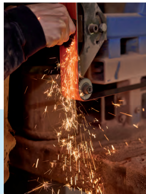
Everett Noel uses a belt grinder to bevel a vegetable cleaver (Summer 2024). Photo by Gabriela Hasbun.
